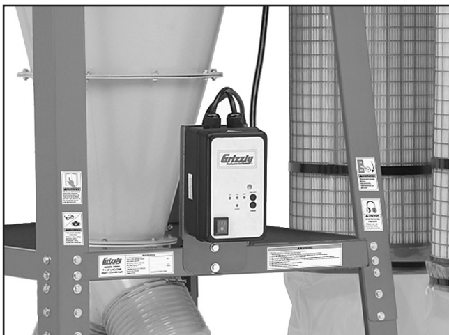
Figure 39. Model G0637 control box mounted.
